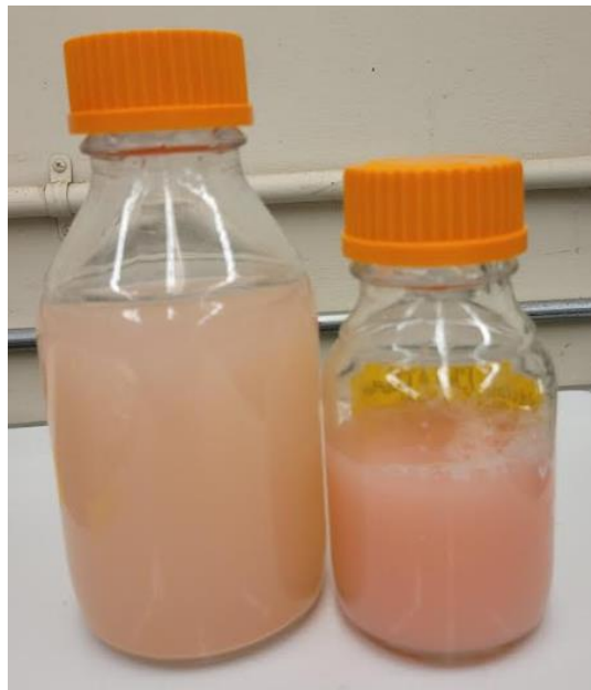
Figure 8.3 The color of H. mediterranei grown on galactose for two (left) and three (right) successive batches at the end of fermentation after 288 hours for each batch.
