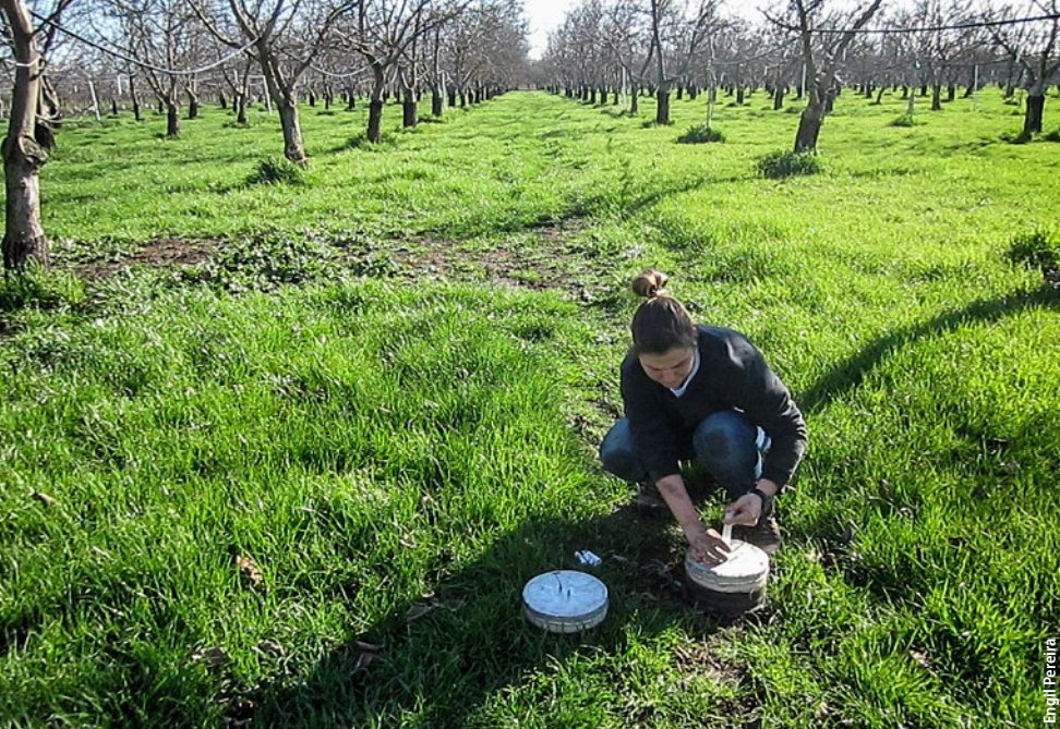
Rafaela Conz, visiting scholar, taking chamber gas samples during gas flux measurements in a walnut orchard.
