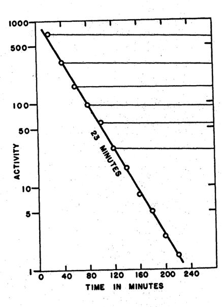
Fig. 5 Result of experiment to show the genetic relation between the 2.3 day and 23 minute substances.
