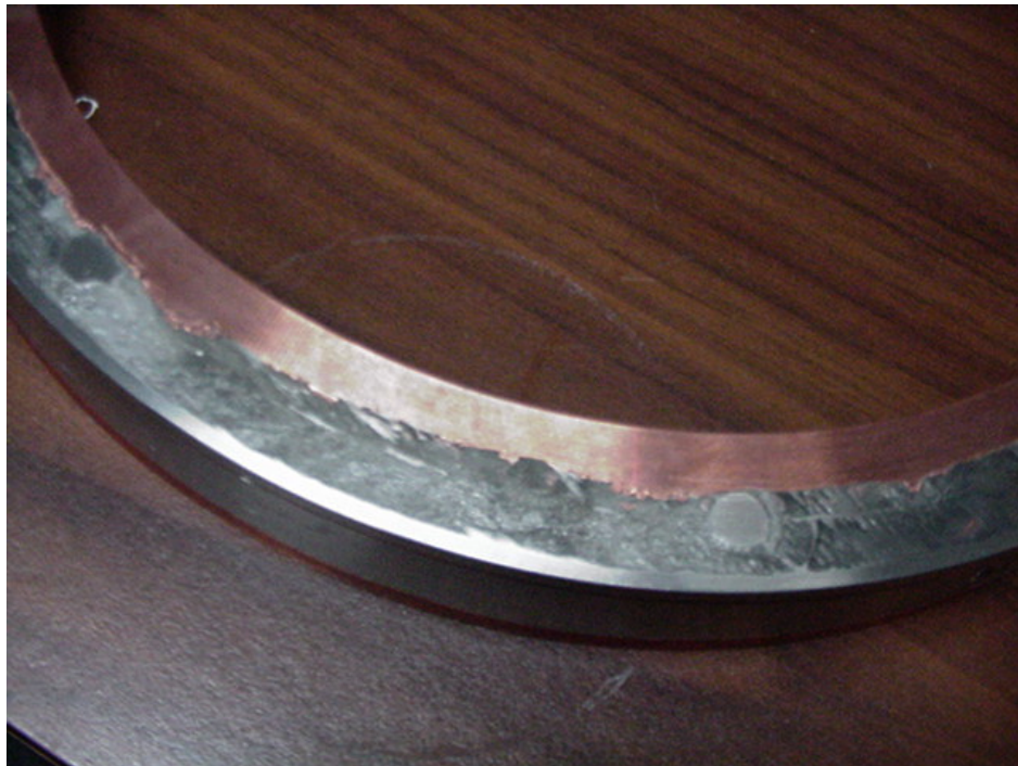
Figure 59. Etching damage in the stainless steel ring.
