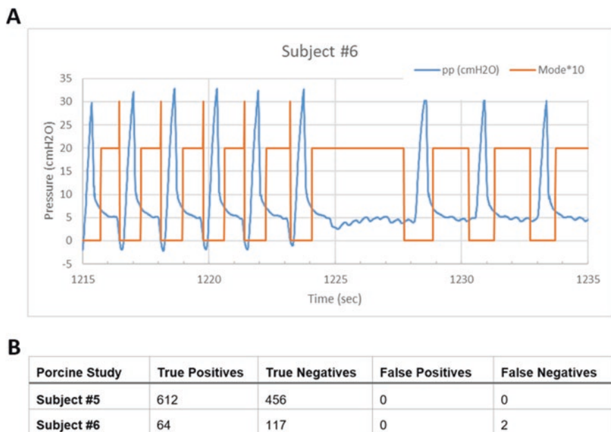
Fig. 15.2 ABBU patient assist mode data in porcine model. (a) A representative trace of pressure data (blue) during the porcine experiment. Mode = 30 means that a patient assist was started, Mode = 0 means that a breath was delivered, and Mode = 20 means that ABBU is calculating PEEP. (b) The test summary of patient assist algorithm on porcine model ( n = 2 )
