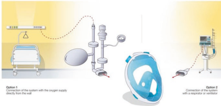
Fig. 23.2 Adaptability of the snorkel mask configuration depending on connection requirements. Image courtesy of Profili et al. [10]
