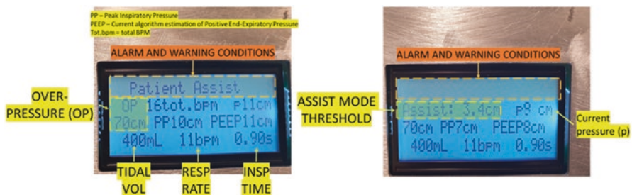
Fig. 12.2 Example of a simple user interface displaying key parameters for ventilatory support
