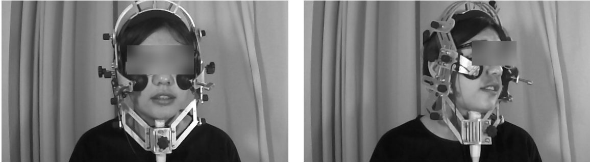
Figure 4.3: Two views of the ultrasound stabilization helmet, ultrasound probe, and microphone (clipped to right cheekpad, most easily observed in image at right) as fit to one participant.
