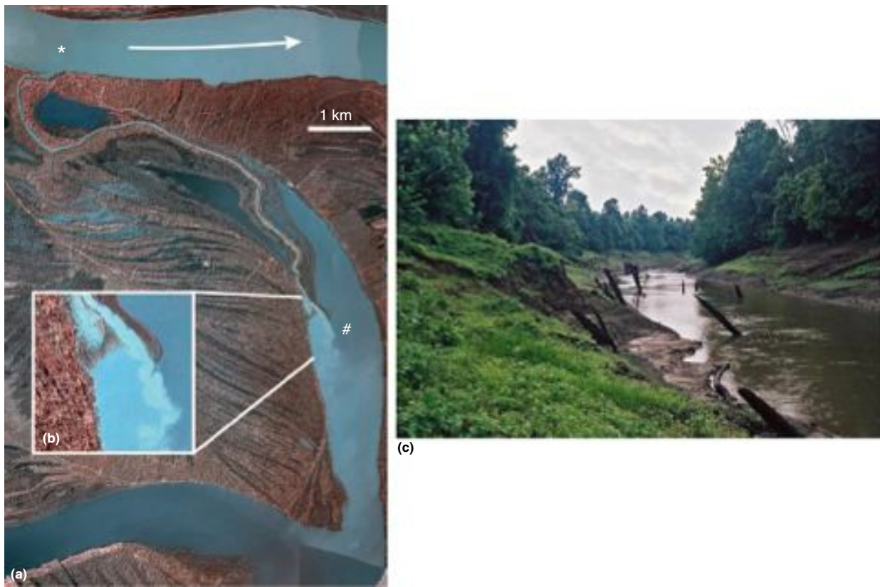
Figure 13 (a) False-color aerial photograph of a tie channel connecting the Raccourci Old River oxbow lake to the Mississippi River (top) approximately 65 km north of Baton Rouge, Louisiana, USA. An * marks the channel junction with the river and the # sign indicates the channel terminus in the lake. (b) Enlarged view of a sediment-laden jet entering the lake at the Raccourci Old River channel. (c) A 95 m-wide section of the tie channel one kilometer from its junction with the Mississippi River. The vertical scar in the foreground and the back-rotated tree stumps in the channel mark failure blocks. Reproduced from Figures 1(a), 1(b), and 13 of Rowland, J.C., Dietrich, W.E., Day, G., Parker, G., 2009. Formation and maintenance of single-thread tie channels entering floodplain lakes: observations from three diverse river systems. Journal of Geophysical Research 114, F02013. doi:10.1029/2008JF001073, with permission from Journal of Geophysical Research .
