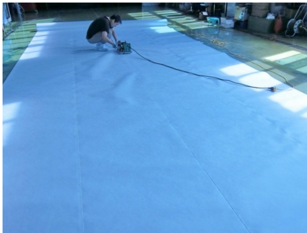
Figure 4.8: The process of making the tyvek reflector.
