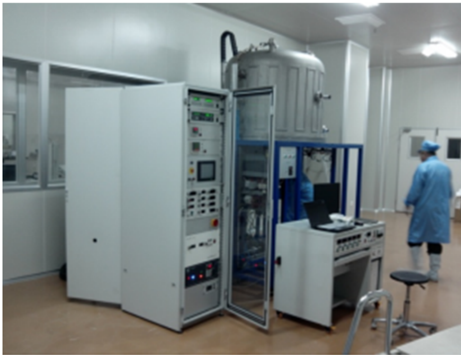
Figure 5.12: Equipment for fabricating 20 inch MCP-PMTs developed by NORINCO using the photocathode transfer technology
