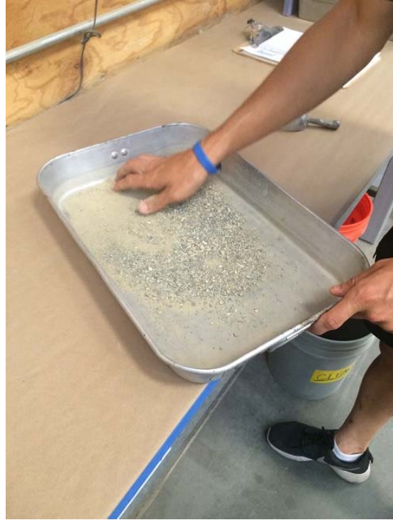
(b) Use a hand to spread the materials evenly, and shake the pan if necessary.
