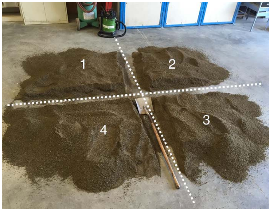
Figure A.3: An example of quartered material on a hard, clean, level surface.
