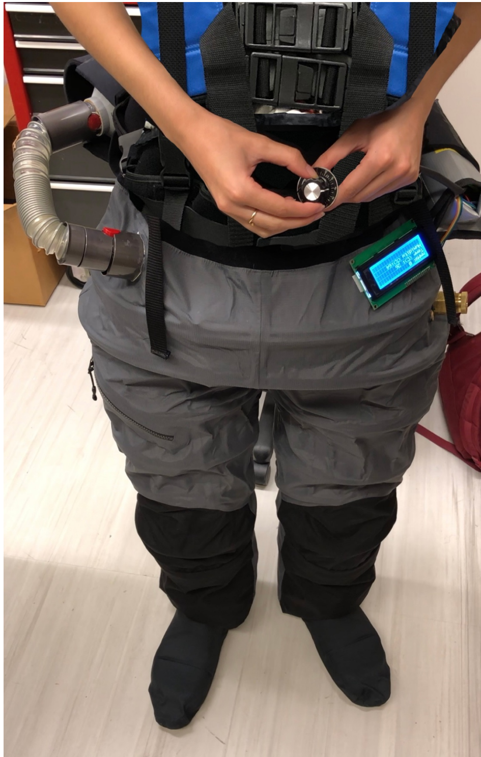
Photograph 2. Mobile Gravity Suit Without Negative Pressure Activation
