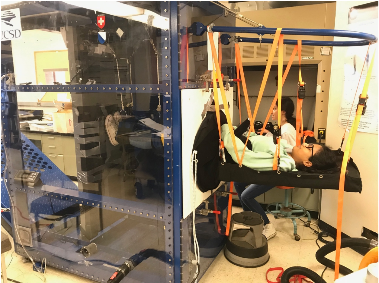
Photograph 1. LBNP Chamber with a user suspended in a supine position.
