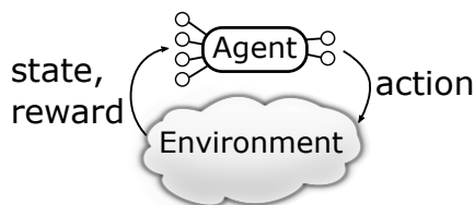
Figure 2.1: The deep reinforcement learning environment-agent cycle. An environment provides state observations and rewards to an agent. State observations are input to a neural network-based policy which decides actions. An agent then makes an action with the goal of maneuvering into states with the highest rewards.
