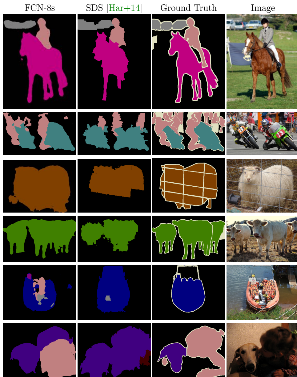
Figure 2.6: Fully convolutional networks improve performance on PASCAL. The left column shows the output of our most accurate net, FCN-8s. The second shows the output of the previous best method by Hariharan et al. [Har+14]. Notice the fine structures recovered (first row), ability to separate closely interacting objects (second row), and robustness to occluders (third row). The fifth and sixth rows show failure cases: the net sees lifejackets in a boat as people and confuses human hair with a dog.
