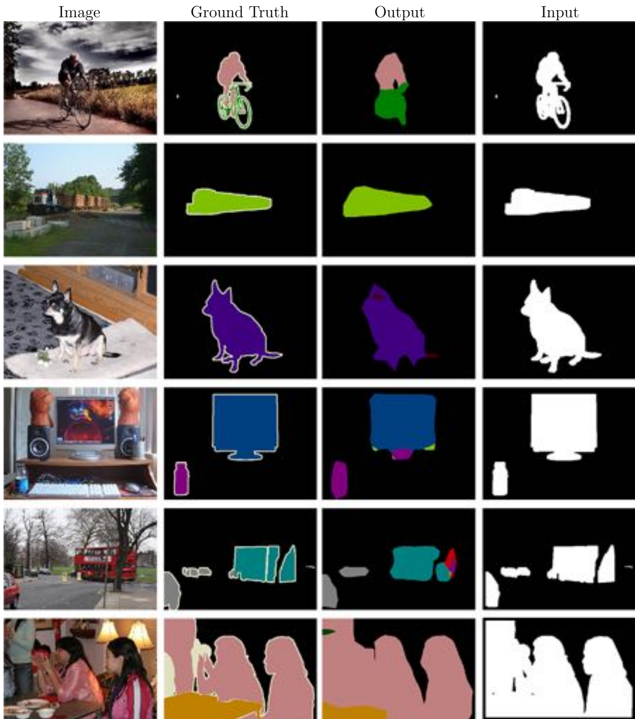
Figure 2.7: FCNs learn to recognize by shape when deprived of other input detail. From left to right: regular image (not seen by network), ground truth, output, mask input.
