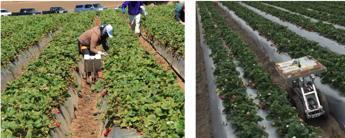
Figure 1. a) Workers picking and transporting trays; b) robot prototype transporting a tray. Photos taken in a strawberry field in Salinas, CA, on August 1, 2017.
