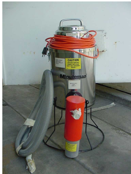
Mercury vacuum cleaner equipped with a mercury separator and a Mersorb™ treated charcoal bed.
