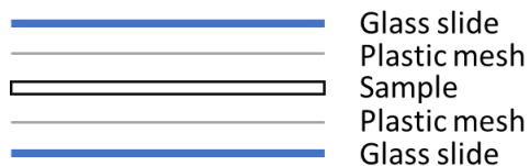
Figure 2.1 The structure of sample during freeze dry.
