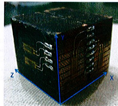
Fig. 5. Strain gages were attached to the Nb 3 Al coil sample, to measure its mechanical properties.
