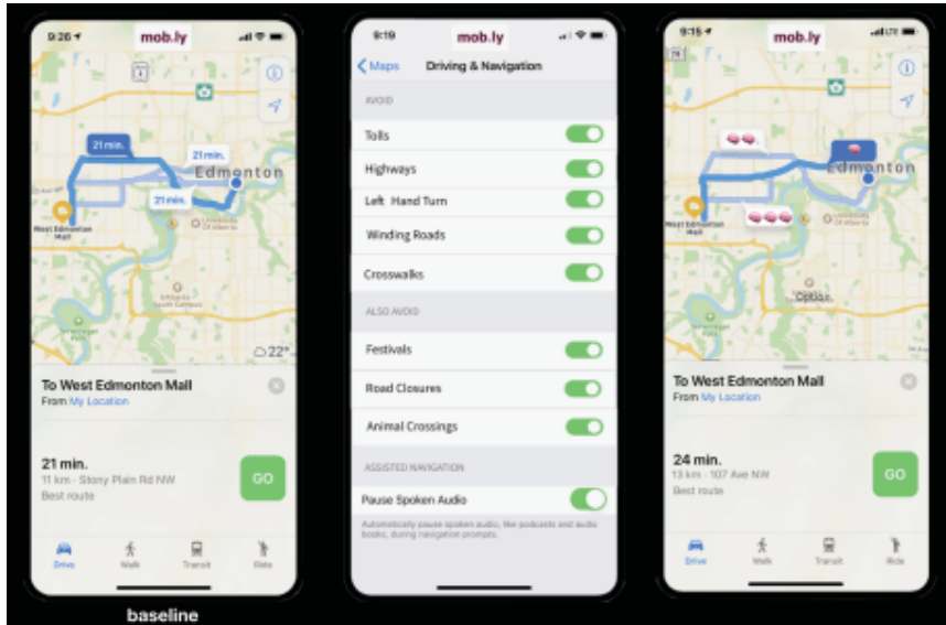
The Mob.ly app interface. (left) Current routing options as determined by an algorithm that minimizes time-to-destination; (middle) Mob.ly allows drivers to select various high-cognitive-load situations they wish to avoid; (right) Mob.ly’s algorithms optimize for low cognitive load.
