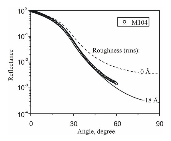
Figure 9: X-ray reflectivity versus angle for the M104 directly polished stainless steel mirror measured at 92 eV. The dashed line shows the theoretical reflectivity of a perfectly smooth mirror and the solid line is a fit to the measurements using a Nevot-Croce factor to model the scattering loss and an rms roughness of 18 Å.
