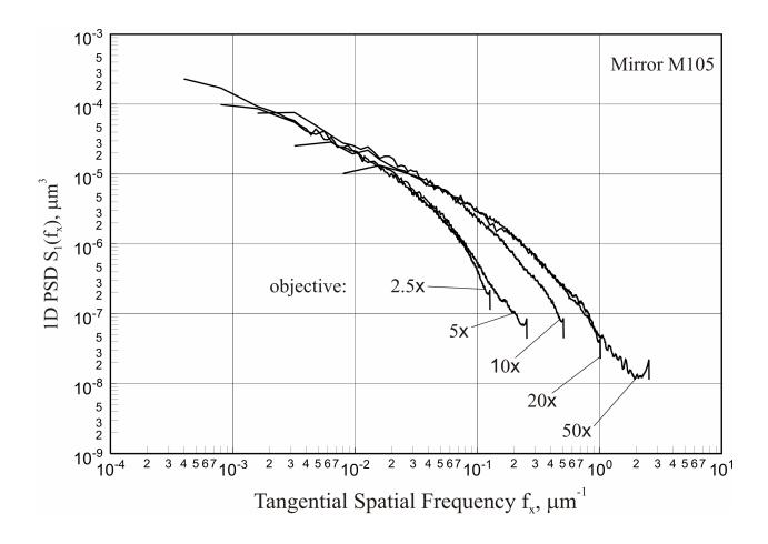
Figure 6: 1D PSD spectra extracted from the 2D PSD distribution of the M105 directly polished stainless steel mirror measured with the Micromap-570 with all available objectives.
