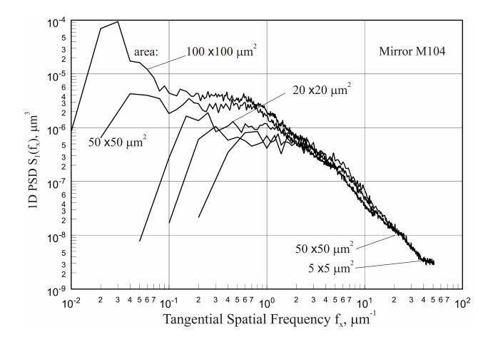
Figure 8: 1D PSD spectra measured with the AFM instrument over different surface area of the M104 directly polished stainless steel mirror. The lowest spatial frequency artifacts are due to the detrending procedure with subtraction of a residual surface described with a third power polynomial.
