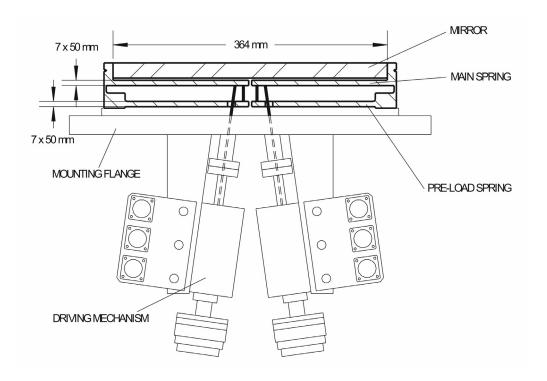
Figure 2: Schematic of flange mounted bending mechanism showing motorized drives, spring/pivot components in ultra high vacuum and the mirror substrate to be bent.
