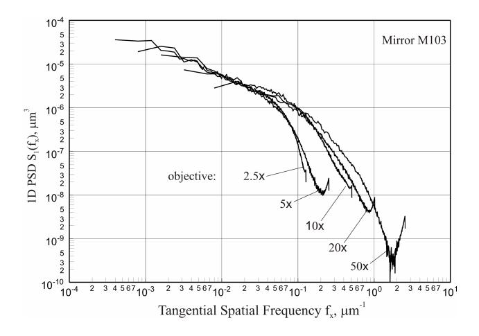
Figure 4: 1D PSD spectra extracted from the 2D PSD distribution of the M103 nickel coated steel mirror measured with the Micromap-570 with all available objectives. Each spectrum is the result of averaging over measurements of five different areas of the mirror surface.
