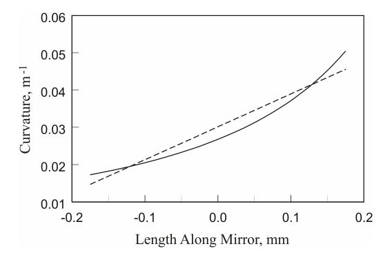
Figure 1: Mirror shape required for perfect focusing, expressed as curvature versus length along the substrate. The dashed line is the best fit achievable with a uniform substrate.
