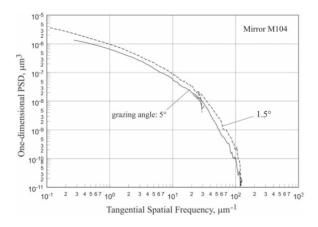
Figure 11: The 1D PSD spectra extracted from the X-ray scattering measurements with the M104 directly polished mirror. The solid line corresponds to the X-ray beam grazing incidence angle of 1.5°; and the dashed line obtained at the beam grazing angle of 5°. The measurements were performed at photon energy of 92 eV.
