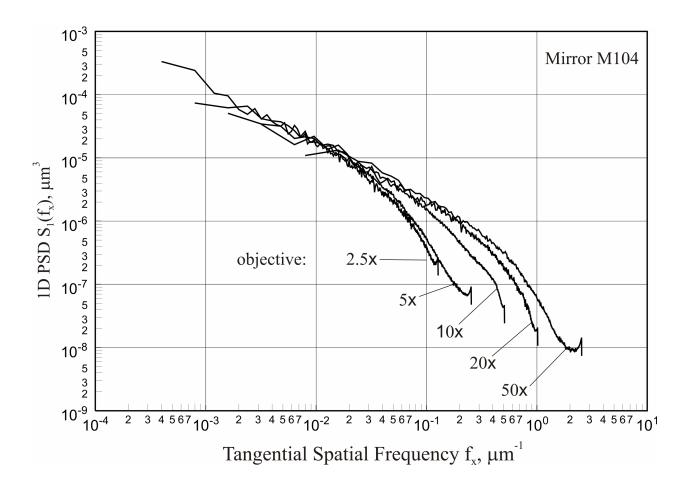
Figure 5: 1D PSD spectra extracted from the 2D PSD distribution of the M104 directly polished stainless steel mirror measured with the Micromap-570 with all available objectives. Each spectrum is the result of averaging over measurements of five different areas of the mirror surface.
