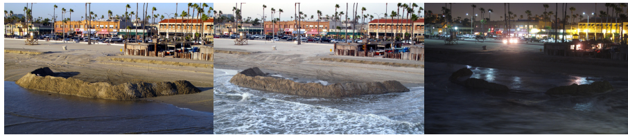
Figure 3.4: Photographs of Berm 2 at (left to right) 17:00, 18:00, and 18:30 shows the progressive rise of the tide and erosion of the berm that occurred in each of the three experiments.
