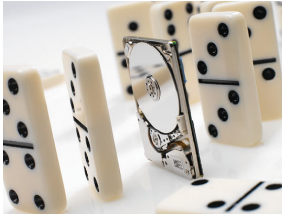
Figure 1.1: 0.85 inch form factor hard disk drive compared to a set of dominos (source Toshiba [7])
