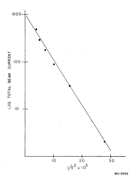
Fig. 16 Total Current Versus Energy, Coulomb Losses (E is energy of Accelerating Electrode)
