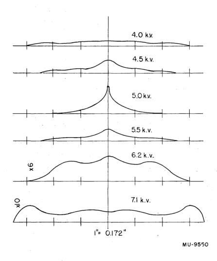
Fig. 9 Beam-Intensity Cross Sections, Variable-Focus Electrode Voltage
