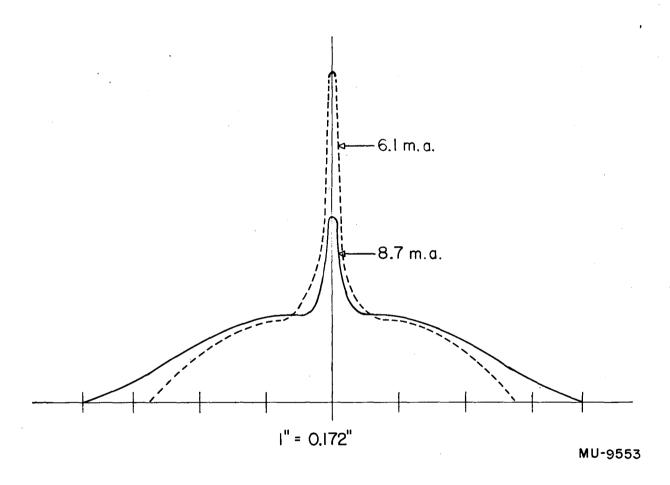
Fig. 12 Beam-Intensity Cross Sections, Space-Charge Effects
