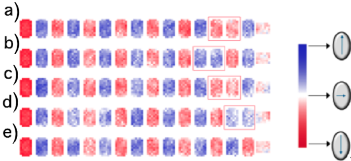
Figure 2.4: Defect diffusion in nanomagnet chains. a)-e), Micromagnetic simulation of the magnetization of a line of nanomagnets with a defect pair highlighted in the first 4 frames. A hard axis field is held at a fixed value of 37 mT. The magnetization of the first nanomagnet on the left is held fixed as an input to set the antiferromagnetic ordering of the chain. A defect that has formed in the wire moves in a random walk until exiting the chain to the right in e).
