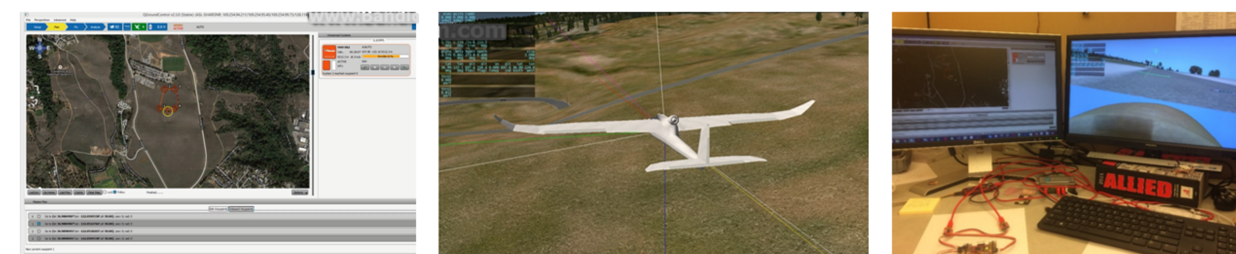
Figure 3: Hardware in the loop (HIL) of single UAV with QGC and X-Plan simulator
