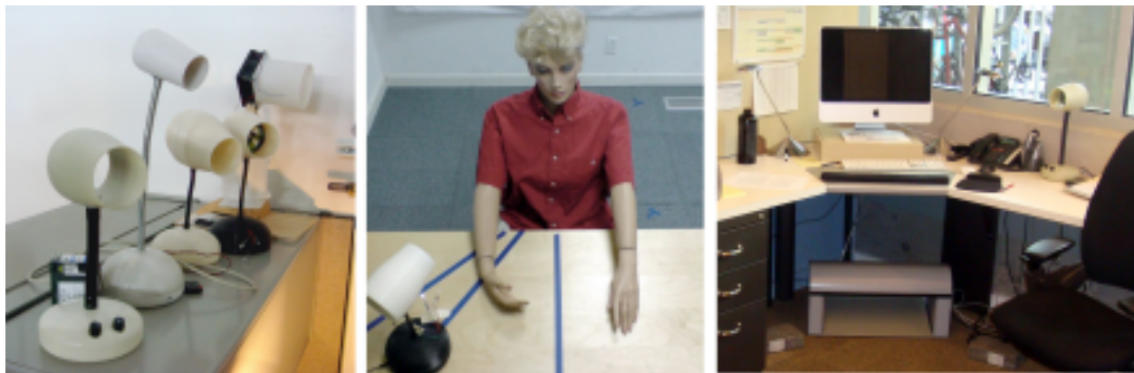
Figures 6a-c. Various fan prototypes, cooling performance test with thermal manikin, and the integrated footwarmer and fan installed in a field study site.
