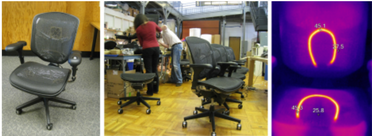
Figures 7a-c. Early heated/cooled chair prototype, fabrication of final design for field research, and thermal camera image with heating elements activated.
