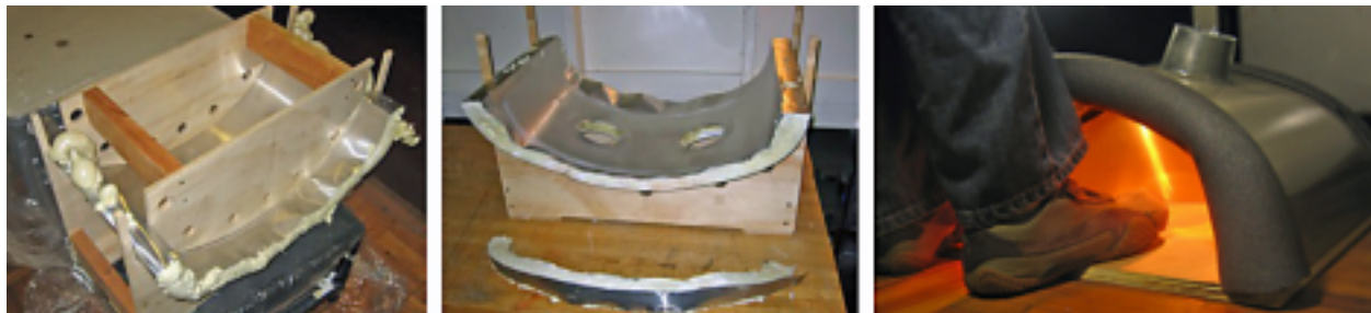
Figures 3a-c. Early prototype for half-ellipse footwarmer, in fabrication and in use. Source: Fannon 2015.
