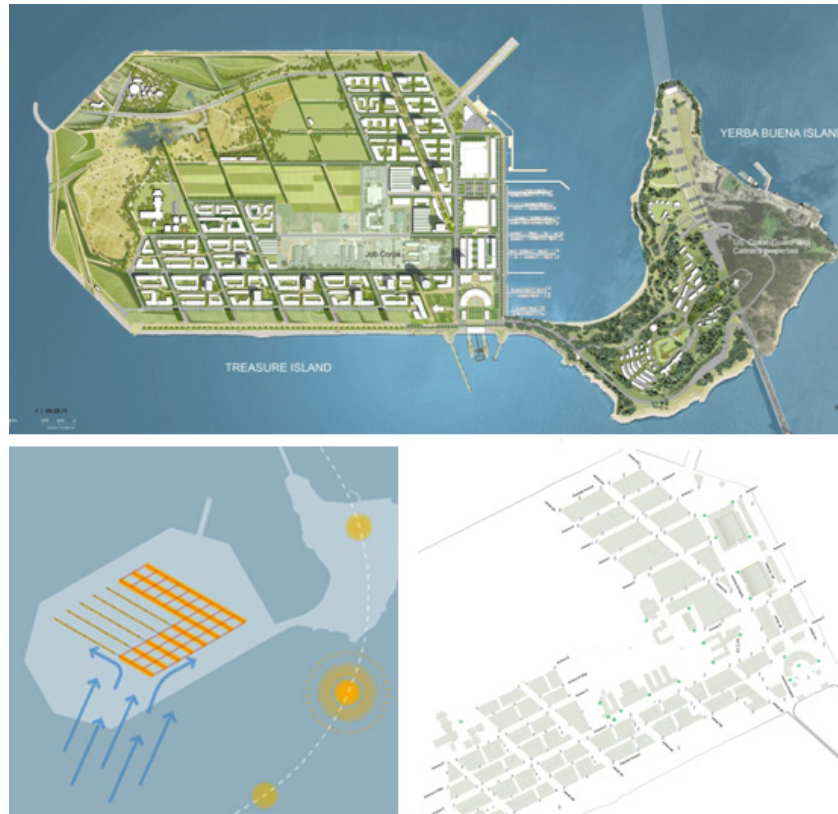
Figure 21. Wind planning of Treasure Island Redevelopment Plan (Sources: San Francisco Planning Department (2011, p. IV.I.39–IV.I.41); Treasure Island Development Authority (2011, pp. 4–5, 18))
