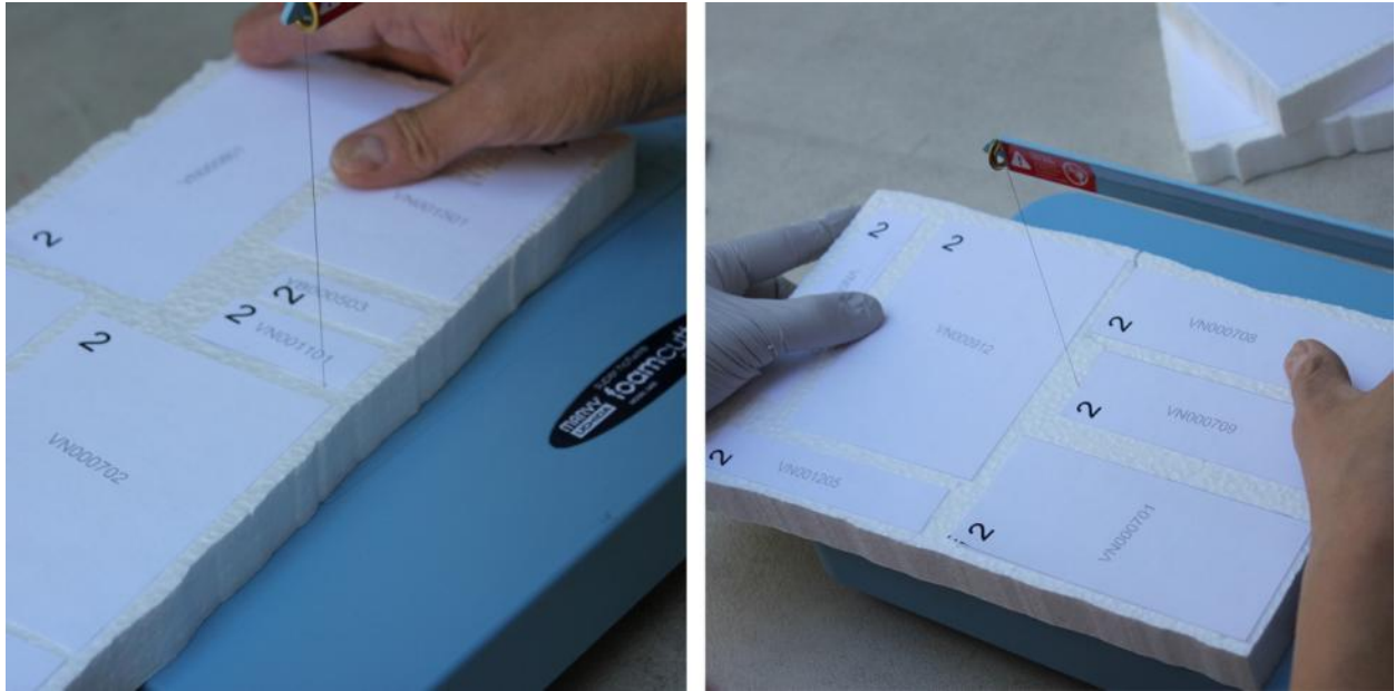
Figure 40. Cutting foam sheet with a hot wire foam cutter.
