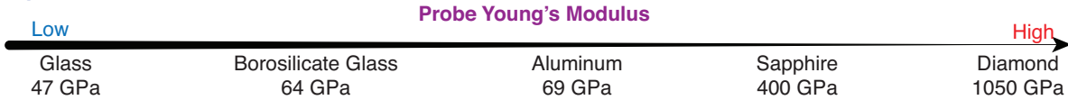
Figure 15 - Part I: Framework provides a guideline for selecting a nanoindentation probe (geometry, size and material). The tip geometry is important to indentation testing; for example, sharp probes are preferred to use on stiff materials to maximize spatial resolution, while blunt probes are preferred to use on soft materials to avoid sample puncture and facilitate sample detection. However, the use of blunt probes comes at the expense of spatial resolution. As for tip material, there is a variety of materials to choose from when testing soft materials and many researchers might choose a tip material that mitigates adhesion and is cheap and easy to manufacture rather than the traditional diamond probes.
