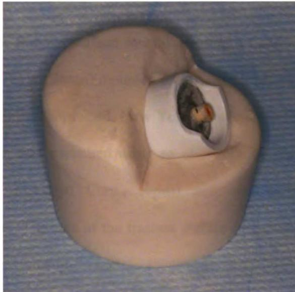
**Figure 4. Mounted specimen in the acrylic jig**
