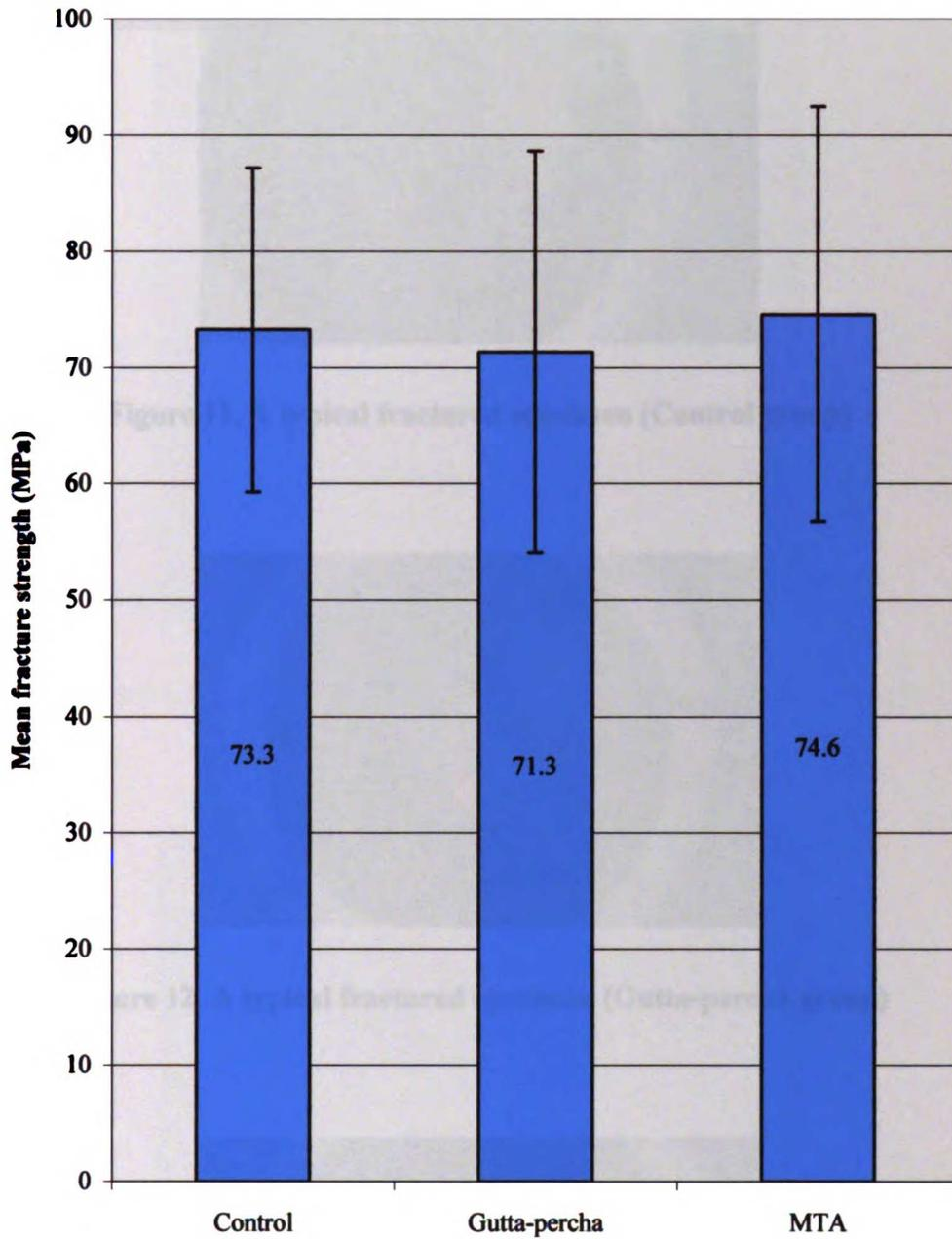
**Figure 10. Fracture strength in MPa (Vertical bars = standard deviation)**
