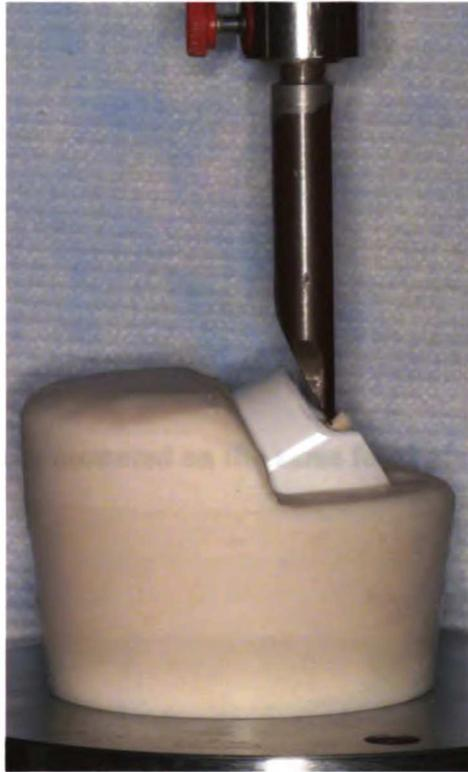
**Figure 5. Fracture strength testing using the mechanical testing machine**
