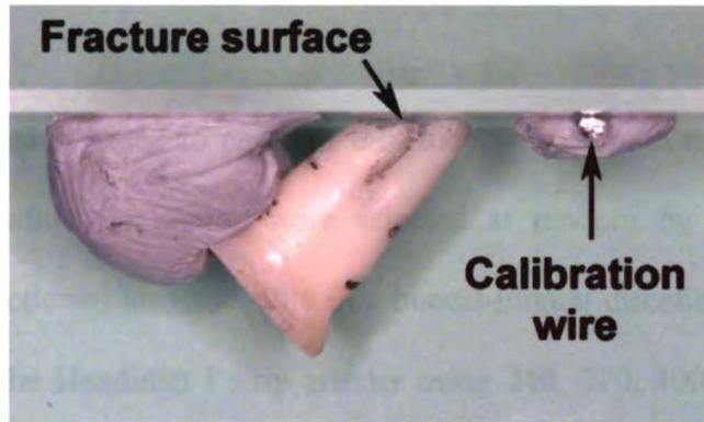
**Figure 7. Fractured surface mounted on the same focal plane as the calibration wire**
