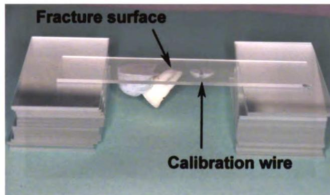
**Figure 6. Fractured specimen mounted with the calibration wire**
