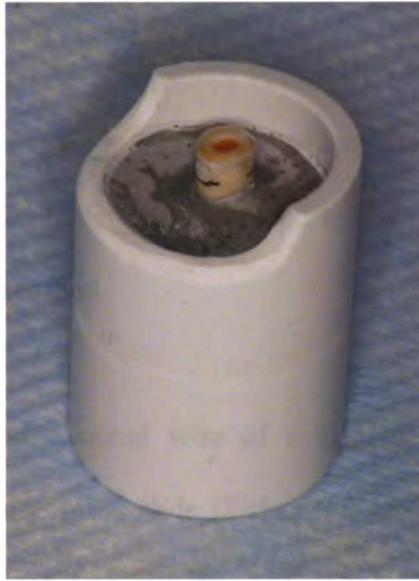
**Figure 3. Specimen mounted in Rockite and PVC coupling**
