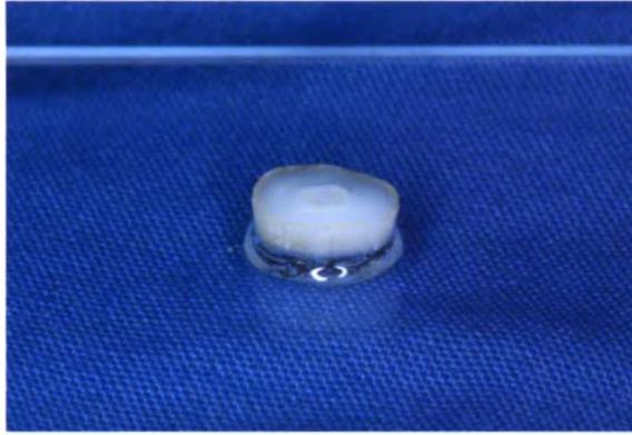
**Figure 9. Specimen mounted for microhardness testing**
