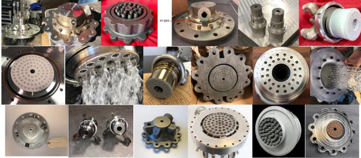
Figure 1.13: Additively-manufactured (L-PBF) LRE injectors for a range of thrust classes, printed and hot-fire tested at NASA MSFC. From NASA MSFC.
