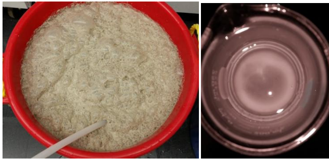
Figure 4-9. Impact of impurities in gypsum on appearance of seed slurry in Gypsum 4, USA Gypsum (left) compared to high-purity Gypsum #5, USG (right)
