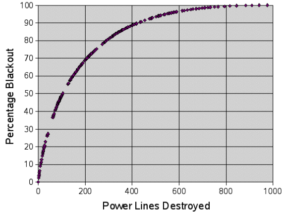
Figure 1: Inhibiting bisection analysis of the Western states grid with integer programming
