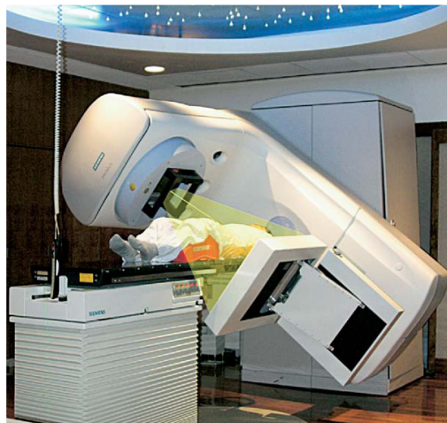
Fig. 1. MV CBCT imaging system using a conventional linac and a flat-panel EPID adapted for the detection of MeV photons. In 45 seconds, the gantry rotates 200^\circ around the patient acquiring one image per degree. The shift required to register the daily MV CBCT with the reference planning CT is available approximately 3 minutes after the beginning of the image acquisition.
