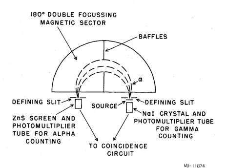
Fig. 2. Schematic diagram of high-geometry spectrograph setup for alpha particle-gamma ray coincidence experiment.
