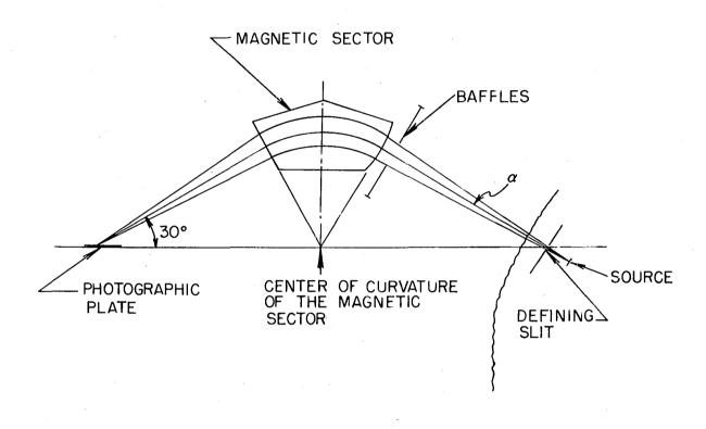
Fig. 1. Schematic diagram of low-geometry spectrograph.
