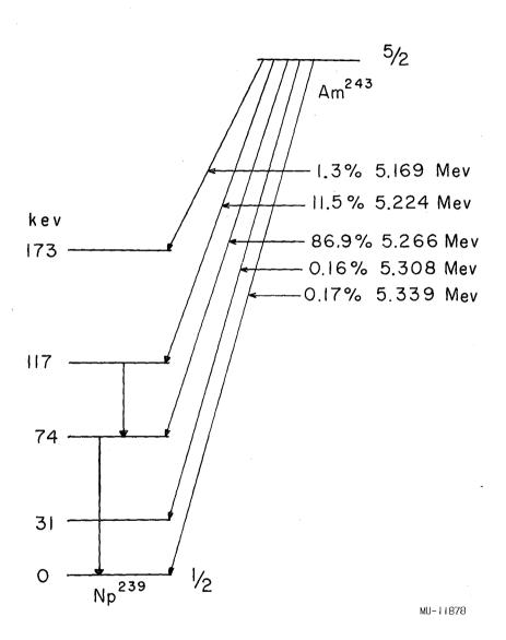
Fig. 7. Decay scheme of  $Am^{243}$ .
