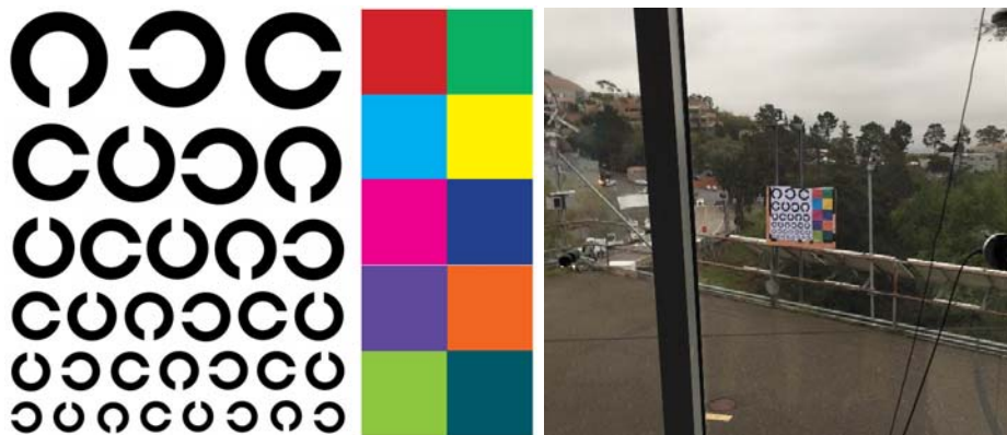
Figure 2. The testing panel (left): Landolt-C vision testing chart and a reference color palette. A view (right) to the panel from the chamber
