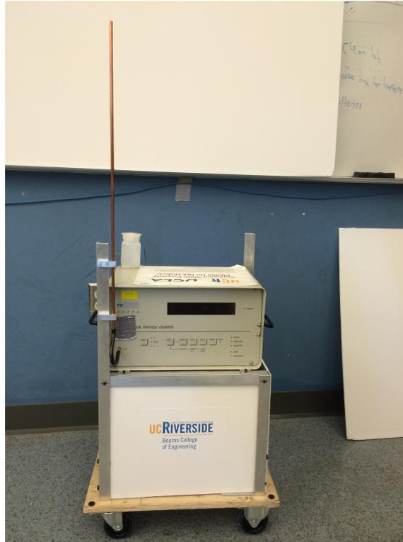
Figure 3.16: Condensation particle counter.
