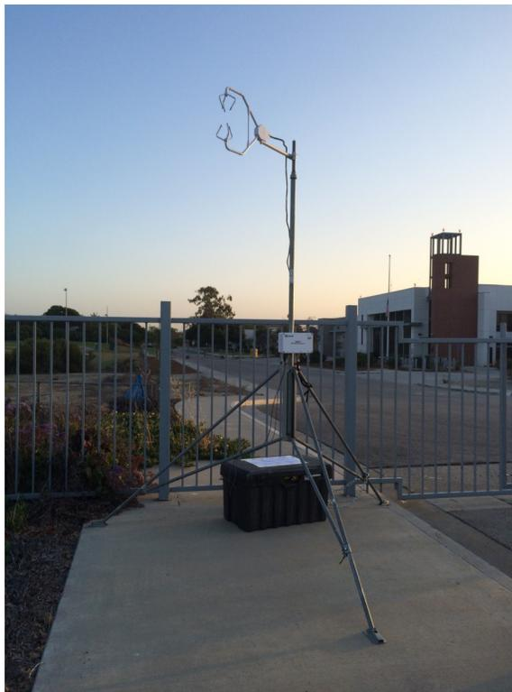
Figure 3.15: Campbell scientific CSAT3 sonic anemometer.
