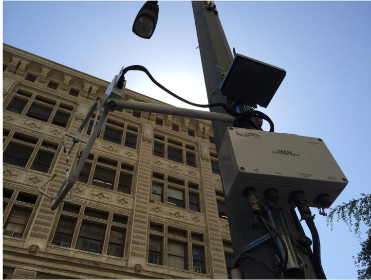
Figure 3.19: Sonic anemometer and AQMesh monitor mounted to light pole next to 8th St.
