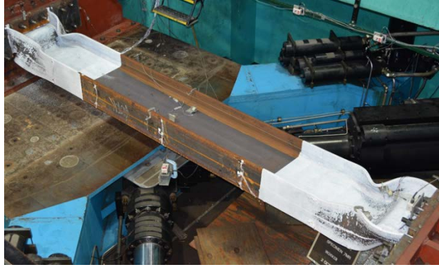
Appendix A22 Group 7 Buckling Mode (W24×131)
