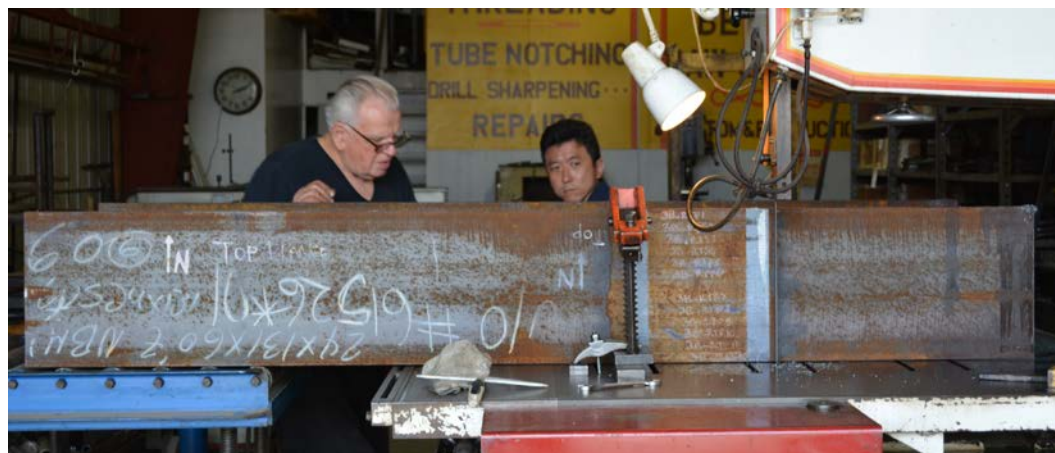
(a) Saw Cutting (Partial Sectioning)
