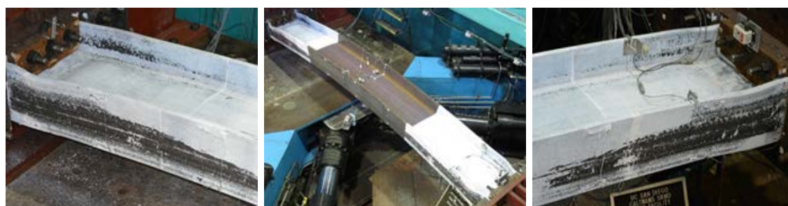
(b) Type S: Single-Curvature Out-of-Plane LTB ( C_a = 0.6 )
