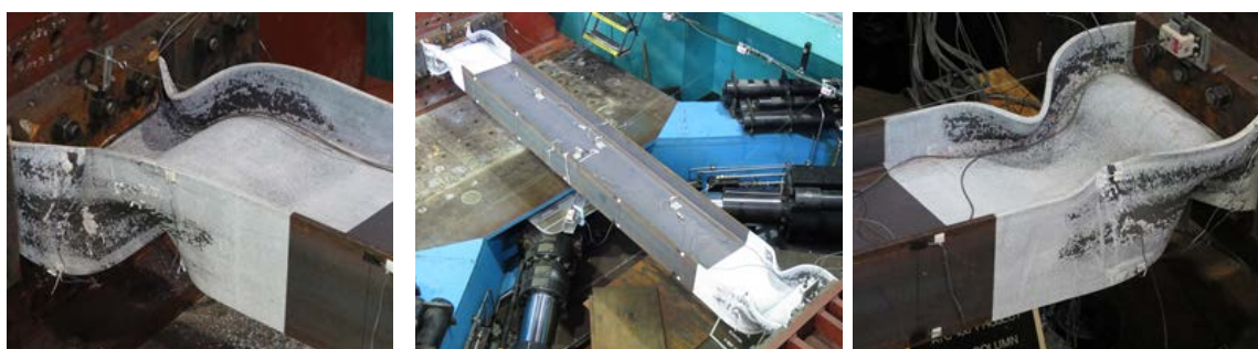
(b) Type D: Double-Curvature Out-of-Plane Movement ( C_a = 0.2 )
