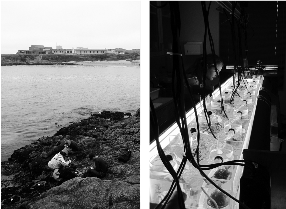
PLATE 1. Field surveys and experimental chambers used to examine the effects of change in seaweed diversity on nitrate uptake and photosynthetic rates: (left) intertidal surveys; (right) chambers arrayed in the chilled water jacket. Photo credits: (left) Bruce Nyden; (right) M. E. S. Bracken.
