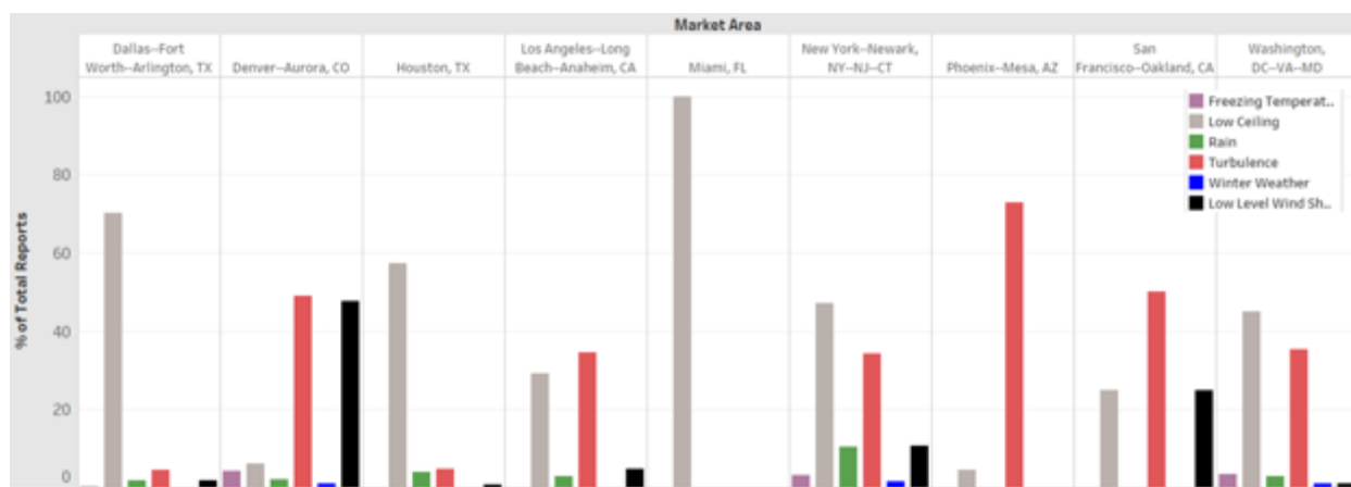
Figure 30: Distribution of PIREPs by weather condition at focus urban areas. No PIREPs were generated across our historical period in Honolulu
