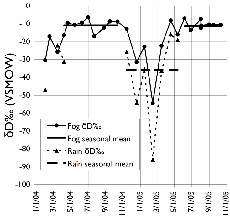
Fig. 8. Isotopic composition of fog and rain water at Site 7. “Fog” values for rainy months are a mixture of fog and rain water. Dry season fog water is consistently enriched compared to rainy season fog/rain water. Horizontal lines are seasonal means (volume-weighted after 11/1/04).
