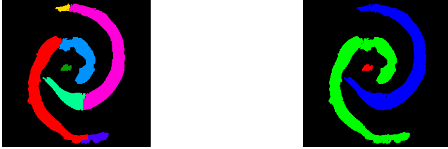
Figure 3.14: Pixel clusters before (left) and after (right) a secondary merging step performed after the main pixel clustering. The secondary merging step joins clusters that are compatible with the same logarithmic spiral arc, but were not previously merged because logarithmic-spiral compatibility was not clear in an earlier stage of the clustering (before near-final cluster shapes were known), or because there was a small gap in the orientation field (these gaps are usually meaningful, but can be jumped over if justified by sufficient compatibility in the near-final logarithmic spiral arc fit). Cluster colors differ between images so that pixel-to-cluster memberships (and cluster merges) are easily visible.
