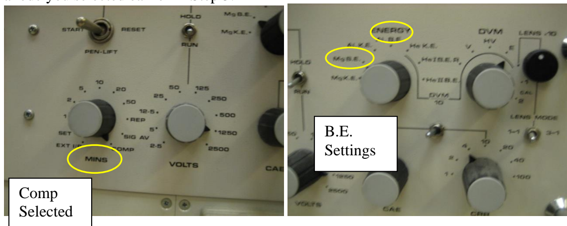
Figure E-9 XPS control panel.
