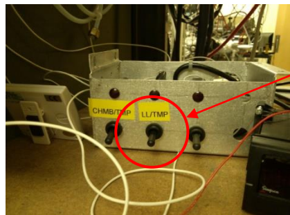
Figure I-5 Pneumatic gate valve control for gate valve between ion gun and top turbo pump.
