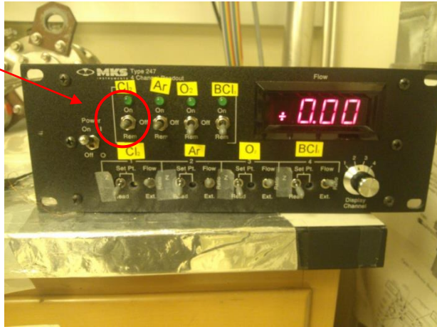
Figure I-7 MFC with Ar gas line switch.
