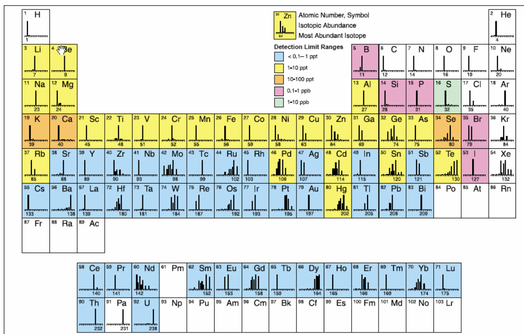
Figure 2-38 Approximate detection capabilities of the ELAN 6000/6100 quadrupole ICP-MS (Wolf 2005).
