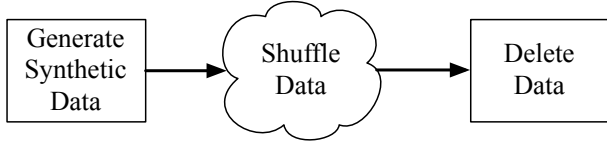
Figure 3: The NetBench application-level benchmark measures the network performance of the entire cluster with an all-to-all shuffle without involving storage devices. Figure reproduced from [5].
