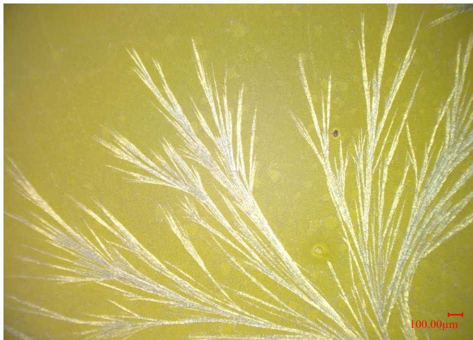
Figure 7.8 Large scale optical micrograph of \text{CH}_3\text{NH}_3\text{PbI}_3 perovskite film exposure for 4 hours in ambient condition spun with LiTFSI
