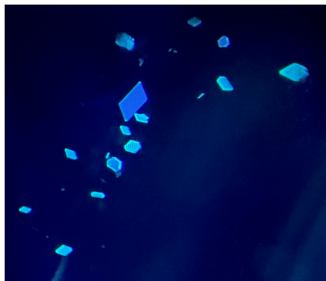
Figure 1. Photograph of crystalline plates of blue luminescent β-Au 2 (μ-dppm) 2 Br 2 ·2CH 2 Cl 2 (1) and teal luminescent blocks of ionic [Au 2 (μ-dppm) 2 Br]Br·2CH 2 Cl 2 (2) taken under UV irradiation.
