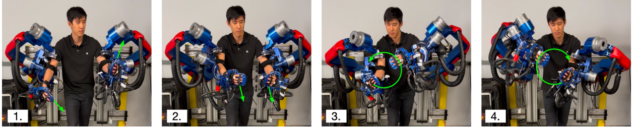
Figure 7.6: Subimages show keyframes of the bimanual interaction with a virtual object. The object is not explicitly defined by its geometry, but rather as a constraint on the total joint space in which the relative pose between the hands is fixed. During keyframe (1), the hands are unconstrained ( \gamma = 0 ). In keyframe (2), the constraint is activated by setting \gamma = 1 . Subsequent motions (2)-(4) show that the virtual rigid coupling between the hands gives the illusion of interacting with a virtual rigid object that can be freely manipulated.
