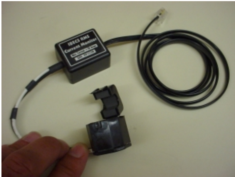
Figure 15. IBECS RMS Current Monitor
