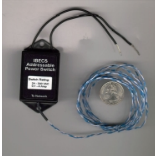
Figure 13. IBECS Addressable Power Switch
