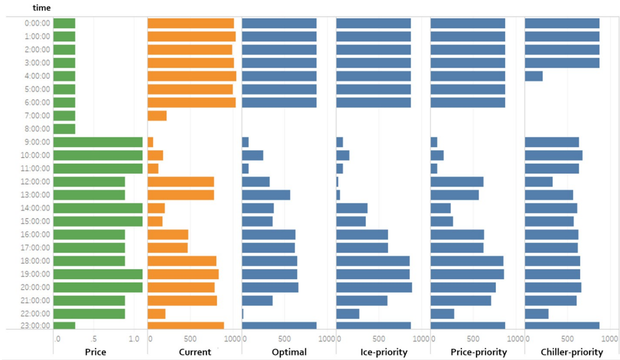
Figure 15 Electricity consumption of different control strategies under the maximum-load scenario
