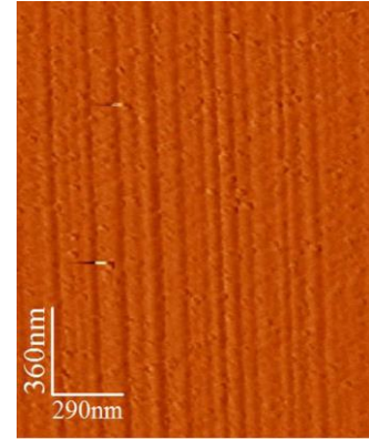
Fig. 9. AFM image of the test sample over a 0.1 \mu\text{m}^2 area, using phase contrast.
