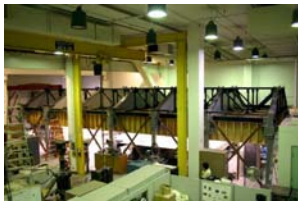
Seismic test structure (left) and scaled building model (right).
