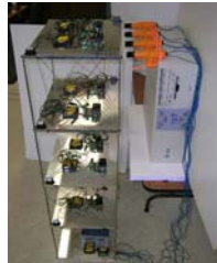
Seismic test structure (left) and scaled building model (right).
