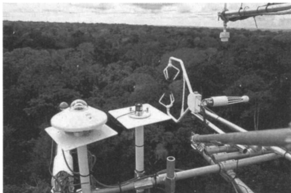
PLATE 1. Eddy covariance tower (height = 64 m) at km83, Tapajós National Forest, Pará, Brazil. Photo Credit: Marcy Litvak.
