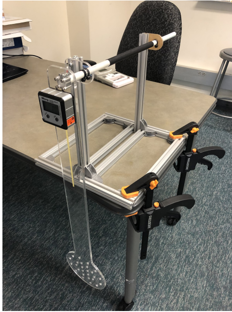
Figure 4.1: Rotatable mock endoscope
