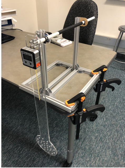
Figure 3.6: Rotatable Mock Endoscope
